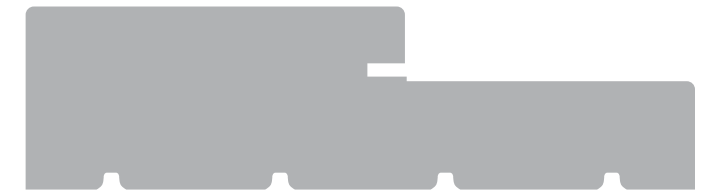
EXTERIOR FRAME WITH A SAW KERF.
