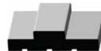
Standard Flat Jamb with Applied Stop
