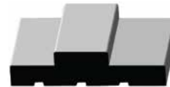
Standard Flat Jamb with Applied Stop
