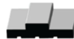
Standard Flat Jamb with Applied Stop
