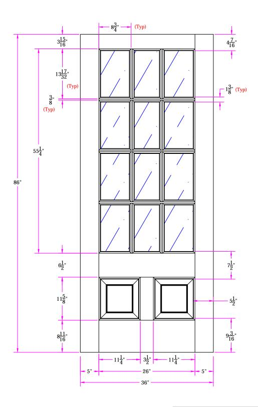
THIS DRAWING AND THE INFORMATION CONTAINED HEREIN IS THE PROPRIETARY TO SIMPSON DOOR COMPANY AND SHALL NOT BE REPRODUCED, COPIED OR DISCLOSED IN WHOLE OR PART, OR USED FOR MANUFACTURE OR FOR ANY OTHER PURPOSE WITHOUT THE WRITTEN PERMISSION OF SIMPSON DOOR COMPANY.
